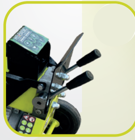
Two-level control system
