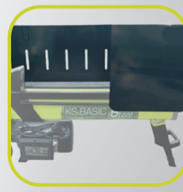
Protective metal cover
